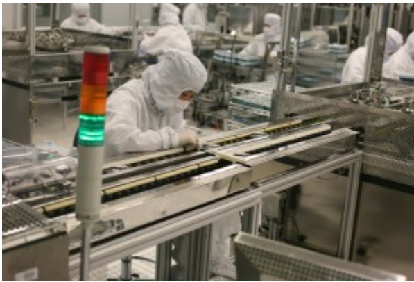
Figure 2.10. Assembly of notebook hard drives in Seagate's "clean room." Wuxi China ( Seagate's clean room by Robert Scoble used under CC BY 2.0 licence )
