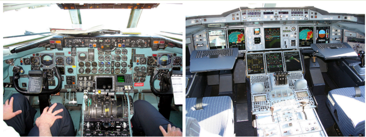
Figure 6.27 Airplane Cockpits. Initial design of the airplane cockpit (left); the digital design of the airplane cockpit (right), which has taken human factors into account.
