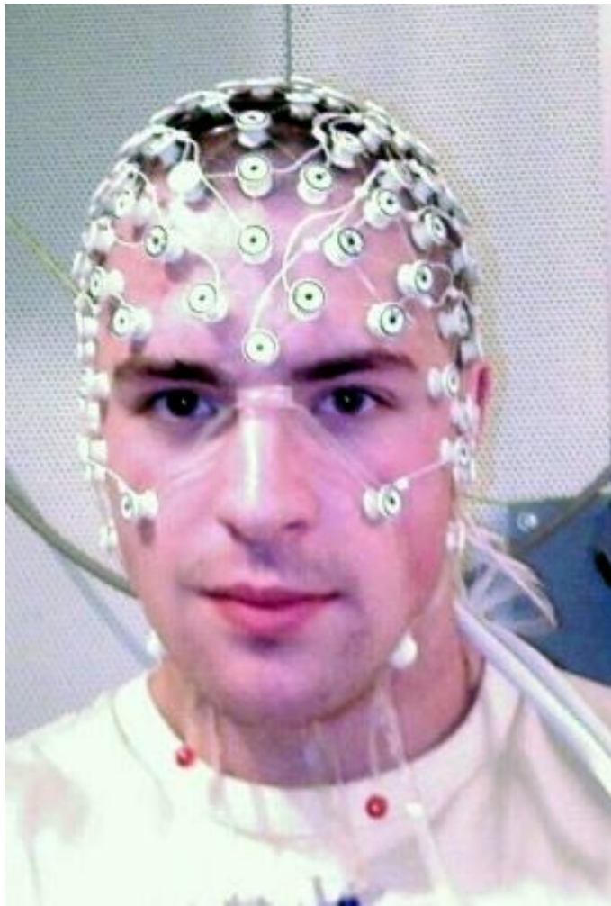
Figure 5.18 EEG Study. A participant in an EEG study with a number of electrodes placed around his head.
