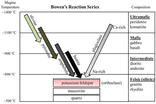
**Figure 3.1** | Bowen's Reaction Series, showing the progression of mineral crystallization as magma temperatures drop from ~1400 °C to ~500 °C. Note the corresponding names for igneous rock composition and some example rock types within each compositional group. Source: Karen Tefend (2015) CC BY-SA 3.0
