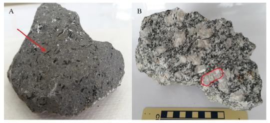
**Figure 3.5** | (A) An example of a porphyritic-aphanitic mafic rock with needle-shaped amphibole phenocrysts (arrow points to one phenocryst that is 1cm in length); No other minerals in (A) are large enough to see. (B) An example of a porphyritic-phaneritic felsic rock with large feldspars (outlined phenocryst is 3 cm length). Surrounding these large feldspars are smaller (yet still visible) dark and light coloured minerals. Source: Karen Tefend (2015) CC BY-SA 3.0
