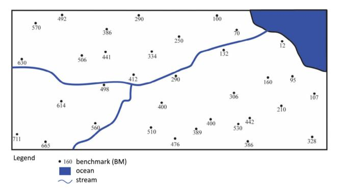
Figure 7-E5 | Elevation measurements and drawing contour maps. Source: Joyce M. McBeth (2019) CC BY-SA 4.0, after Brad Deline (2017) CC BY-SA 3.0
