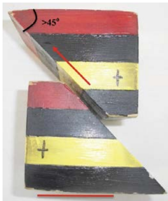
Figure 8.30 / The hanging wall block, at the top, has moved up relative to the foot wall block, at the bottom, resulting in a reverse fault. Note how much closer the cross symbols have become as compared to figure 8.27, evidence for the shortening of the block, due to compression. Also note that the crust has thickened in the region of the fault. Source: Randa Harris (2015) CC BY-SA 3.0. view source .
