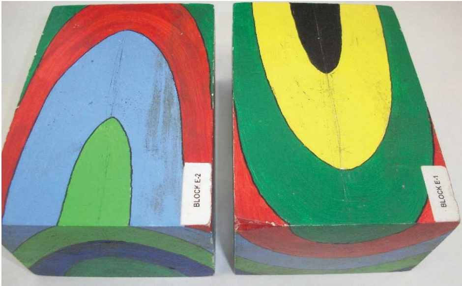
Figure 8.23 | Both blocks are plunging folds. Note the V shape created in map view in a plunging fold. Based on our view of the cross section at the end of the left block, it is a plunging anticline. The fold on the right block is a plunging syncline. Source: Randa Harris (2015) CC BY-SA 3.0. view source .
