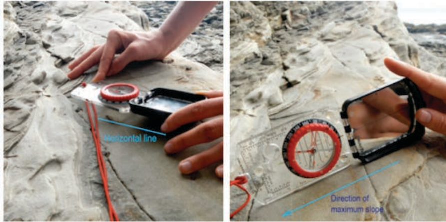
Figure 13.36 Measurement of strike (left) and dip (right) using a geological compass with a clinometer. Source: Steven Earle (2015) CC BY 4.0
