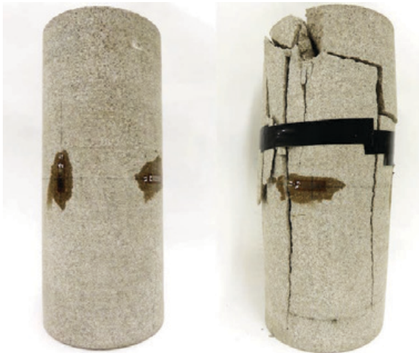
Figure 13.5 Cylinders of rock used to test the strength of rock under compression. The cylinder on the left has been equipped with strain gauges to measure the amount of deformation. The cylinder on the right has undergone brittle deformation after being compressed. Source: Karla Panchuk (2016) CC BY 4.0
