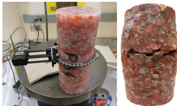
Figure 13.6 Cylinders of potash before and after deformation. The potash underwent ductile deformation before it finally broke. Source: Karla Panchuk (2018) CC BY 4.0
