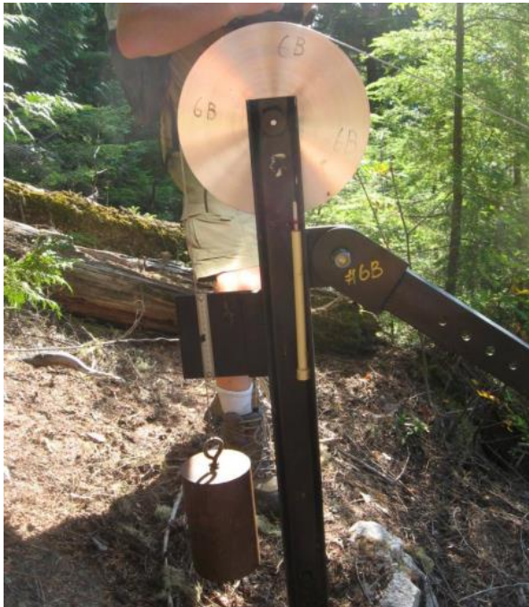
Figure 15.19 Part of a motion-monitoring device at the Checkerboard Slide near Revelstoke, BC. The lower end of the cable (extending out from the top of the device to the right) is attached to a block of rock that is unstable. Any incremental motion of this block will move the cable, which will be detectable by this device. Source: Steven Earle (2015) CC BY 4.0. View source https://opentextbc.ca/geology/
