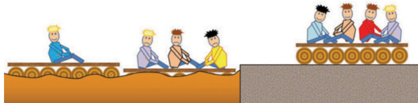
Figure 3.18 Illustration of isostatic relationships between rafts and peanut butter (left), and a non-isostatic relationship between a raft and solid ground (right). Source: Steven Earle (2015) CC BY 4.0
