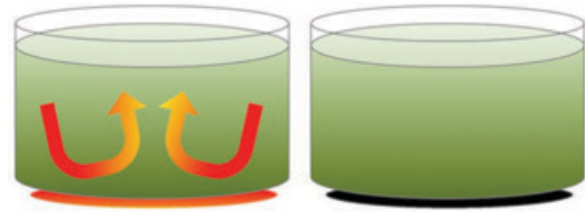
Figure 3.12 Convection in a pot of soup on a hot stove (left). As long as heat is being transferred from below, the liquid will convect. If the heat is turned off (right), the liquid remains hot for a while, but convection will cease. Source: Steven Earle (2015) CC-BY 4.0
