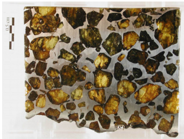
Figure 3.3 Cut and polished slab of a stony-iron meteorite called a pallasite, thought to have formed in a collision that smashed mantle rocks against the metal core of an asteroid early in the solar system's history. Green and brown crystals are the mineral olivine. The metal between the olivine crystals is an iron-nickel mineral. Source: Muséum de Toulouse (2012) CC BY-NC 2.0
