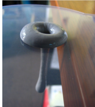
Figure 3.22 Silly Putty exhibiting plastic behaviour when acted upon by gravity over several hours. Source: Erik Skiff (2006) CC BY-SA 2006
